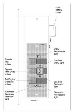
The digital controller provides sensing, timing, and control functions for the ATS. This micro-processor-based controller includes built-in control buttons and status lights for control of the ATS and the generator. PUSH BUTTONS
